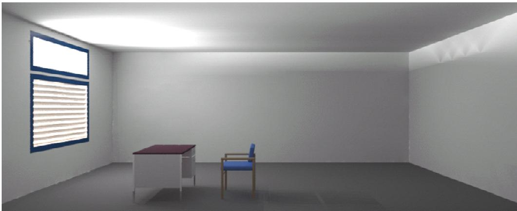
*Figure 4: Photorealistic visualization of room illuminated by standard venetian blinds in the lower facade area and a light redirecting glass in the upper facade area.*
