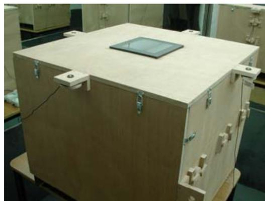
Figure 8. Scale model with the Serraglaze™ sample over the opening surface
