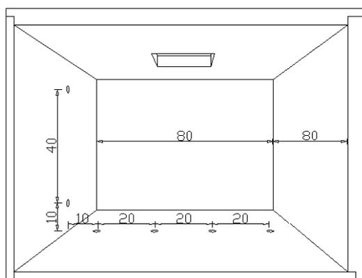
Figure 7. Measurement points positions for the Serraglaze™ scenarii
