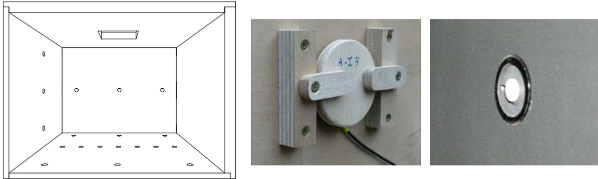
Figure 3. Measurement points locations and photocell positioning system
