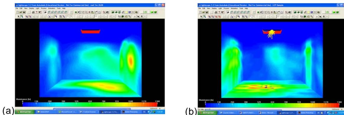
Figure 21. Illuminance distribution obtained by ENTPE method for LCP scenario. (a) shows results with bare opening while (b) shows results with the LCP sample.
