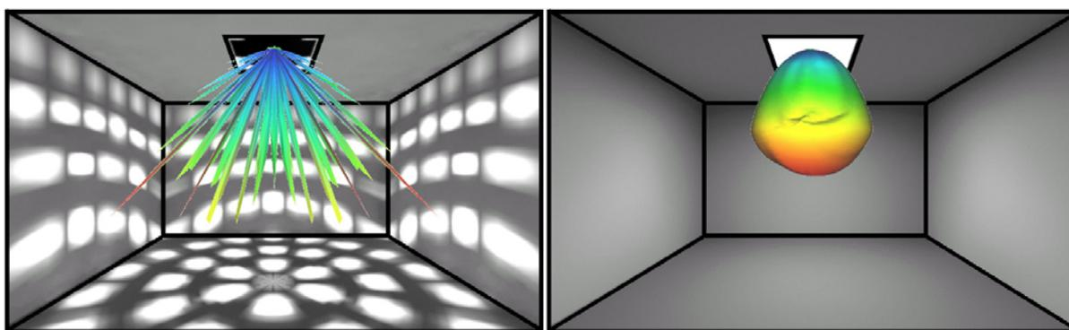
Figure 15. Influence of filter corrections. Left-hand figure: Superposition of the *unfiltered* indicatrices of diffusion. Right-hand figure: Superimposed *filtered* indicatrices of diffusion.
