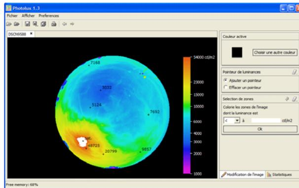
Figure 5. Using calibrated photos to produce a luminance map in Photolux
