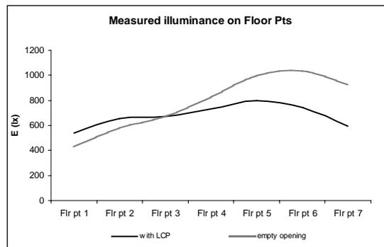
Figure 20. Influence of LCP on the illuminance distribution inside the scale model
