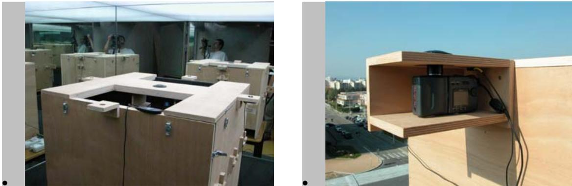
Figure 4. Camera positioning systems for artificial and real sky scenarios
