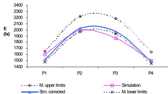
Figure 14. Influence of the near field corrections on the correlation between measurements and simulation results
