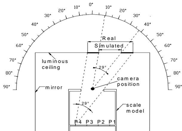
Figure 13. Illustration of the near field error source
