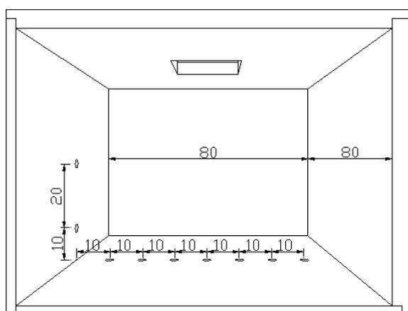
Figure 10. Measurement points positions
