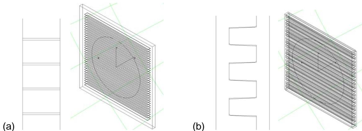
Figure 6. Illustration of the considered complex glazing materials. (a) Laser Cut Panel. (b) Serraglaze™.
